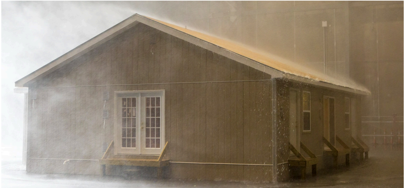
Hurricane-force wind and rain testing at the Insurance Institute for Business and Home Safety (IBHS) Research Center (Photo: Fortified Home)
